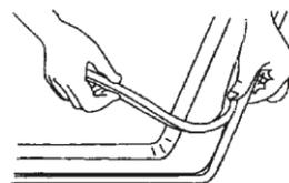
2) Place the gasket around the bottom edge of the hob as shown in the illustration on the right.
