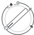
When the knob stops turning and is aligned with the STOP position (see figure), the cycle has finished. Turn off the appliance using the ON/OFF button, and open the door of the dishwasher. Wait a few minutes before unloading the dishwasher to avoid handling the dishes and utensils while they are still hot and more susceptible to breakage. They will also dry better.
