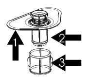
The filter system consists of a filter cylinder (Coarse filter), A flat (Main filter) and a microfilter(fine filter).
