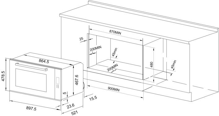
The panels of the adjacent cabinets must be made of heat-resistant material .In particular ,cabinets with a veneer exterior must be assembled with glues which can withstand temperatures of up to  $100^{\circ}$ C. In compliance with current safety standards, contact with the electrical parts of the oven must not be possible once it has been installed.
