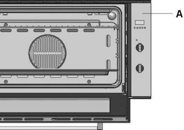
Electronic programmer-Allows you to programme the desired cooking times by selecting the cooking duration and the end cooking time. It can also be used as a timer (only available on certain models)
