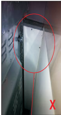
Left Side of oven, chain not attached
