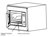
2. Open the door; fix the oven to the cabinet with SCREW at the INSTALLATION HOLE of TRIM KIT. Then fix the TRIM-KIT PLASTIC COVER to the INSTALLATION HOLE.
