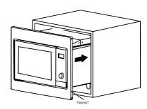
1. Do not trap or kink the power cord. Make sure that the oven is installed in the center of the cabinet.
