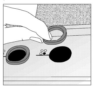
Remove the vitroceramic glass -frame group. Pull and take out the preventive washer at the bottom of the knobs on the vitroceramic glass -frame group.
