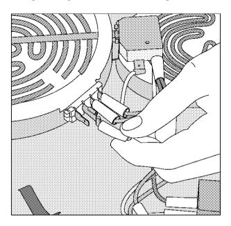
Remove the vitroceramic glass - frame group prior to this operation. Disconnect all the sockets on the vitroceramic hotplate and take the released hotplate.
