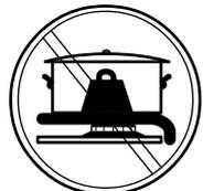
Do not use large pots or heavy weights which can bend the pan support or deflect flame onto the hotplate.
