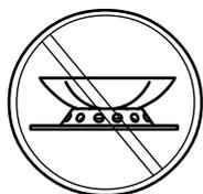
Do not remove the pan support and enclose the burner with a wok stand as this will concentrate and deflect heat onto the hotplate.
