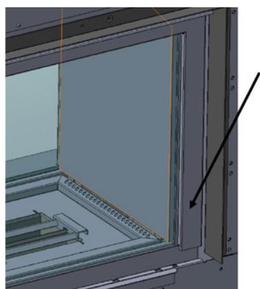
Remove door frame cover (lift up from bottom legs and pull down to remove top from locating tabs.)
