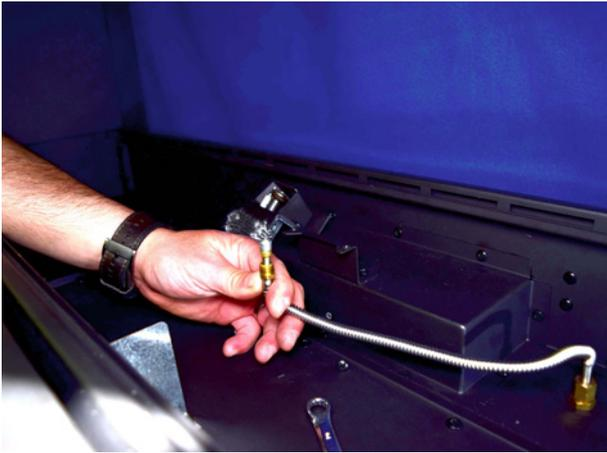
28. Remove injectors from burner. Turn burner over gently. AVOIDING DAMAGING THE INSULATION.2 9.
