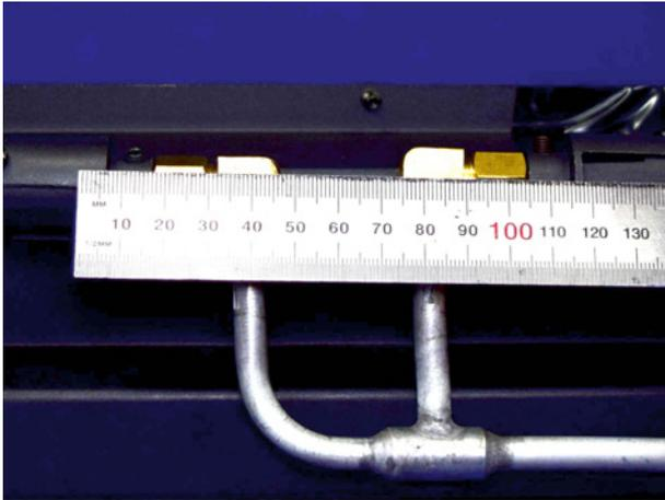
37. Refit gas manifold tube and tighten.
