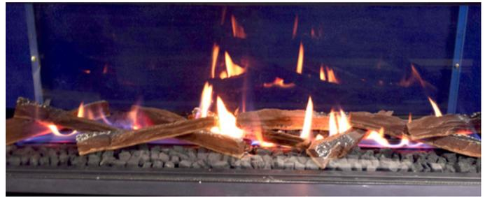
Excessive color (high yellow / orange color and possible sooting on media) – aeration caps require openings to be increased. Check openings as per media table.
