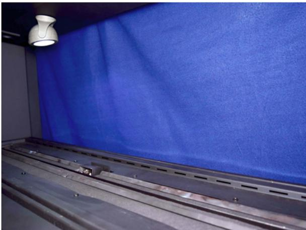
The insulation media can be repainted using an approved high temperature paint, contact Glen Dimplex for details.
