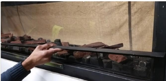
On 1200 models remove the 4 screws holding the lower trim and lift away from door.
