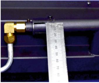
**Note** - A ruler or similar can be used to check the opening, a drill bit of the designated size can also be inserted to check the opening.
