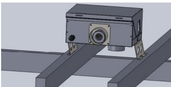
**NOTE** – a minimum of 2m of flue must be run between appliance and fan module.
