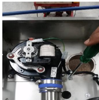
Push fan terminal into position. And affix to wall.
