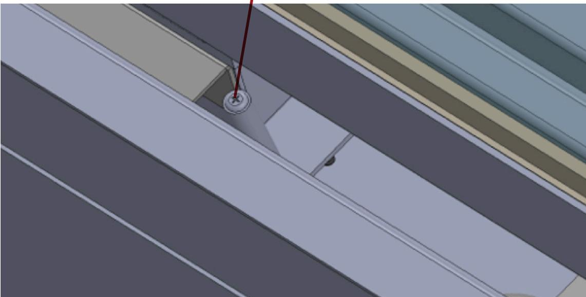
The appliance is supplied with a burner pressure test point located under the lower trim on the gas valve side.
