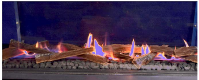
Poor flame color (weak color – very blue flame)- aeration adjustment may requiring further closing or tightening of aeration caps.
