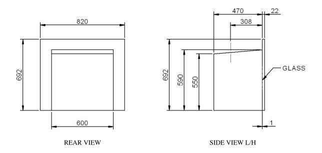
NOTE: Dimensions do not include the insulating blanket. Add 15mm to rear and top to allow for insulating blanket.
