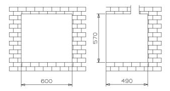
Measure the fireplace recess and remove bricks as necessary to accept the firebox outer case. Clear away any loose rubble and inspect before installing the fireplace.
