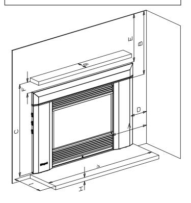
NOTE: Mantel clearances and hearth(floor protector) requirements for Installation listed here are for masonry recess installation.
