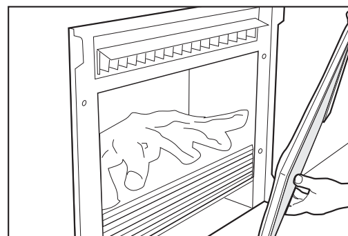
Figure (7) Remove door carefully to prevent damage or breaking of glass.
