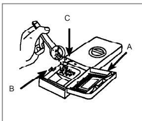
**Notice:** To enable the cover to close, remove any excess detergent from the edges of the dispenser.
