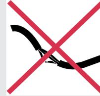
If the power cable wires are frayed or cut
