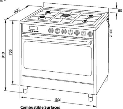
This appliance shall be installed in accordance with AS 5601-2004 - Gas Installations Figure 5.1: Required Clearances around Domestic Cooking Appliances.
