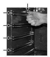
To remove the Oven Shelf Support, push down on the wire below the locking pin, pull away from the oven wall until you can release the bottom of the support from the holes in the oven wall. Replace in reverse procedure.
