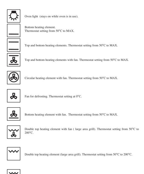
Top heating element (small, low power grill). Thermostat setting from 50°C to 200°C.
