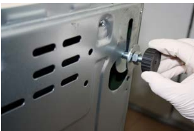
Figure 3. Leg installation on the footstall
