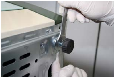
Figure 5. Once the leg is adjusted at the needed height, tighten the nut using a suitable spanner
