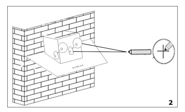
**2)** Position the hood against the wall that you are intending to install it on and mark the position of the screw holes that are to be drilled (as shown in the figure below).
