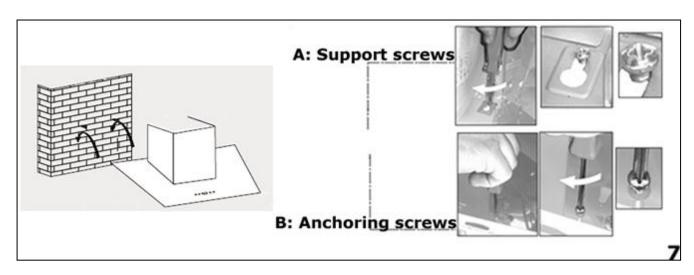
7) Fully tighten the support screws (A) and then screw the anchoring screws (B) through the relevant holes in the cooker hood. Fully tighten the anchoring screws into the wall.
