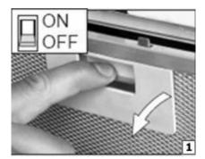
1) Remove the grease filter (as described previously).
